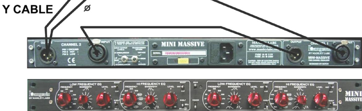
It really is unlikely that simply patching SUM into Left Mix and DIF into Right Mix would ever be useful but the above example might be by virtue of subtlety and L/R separation. Mixing a small amount of DIF into the main path involves less electronics than using SUM-DIF to decode, processing using Inserts 2&3, then re-encoding to Left and Right.
