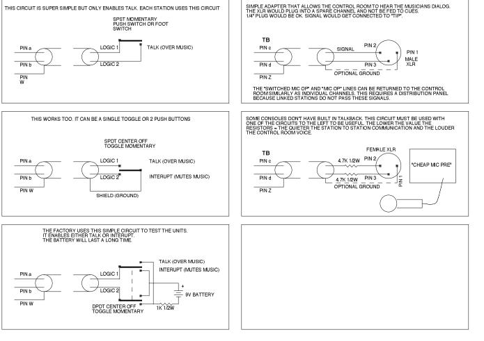
THIS CIRCUIT SHOULD BE USED WITH THE CIRCUIT TO THE LEFT. IT ALLOWS TALK, INTERUPT AND LISTEN.
