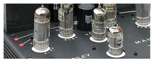
The EL84 tube has quite an interesting history. It was originally developed by Philips in Europe for audio amplification. It soon found its way around the world, being designated as the 6BQ5 in North America. I won't go into an eye glazing, micro history of the tube, but suffice it to say it has proven quite versatile for more than 50 years. It was also put to use by British Invasion bands during in the mid 60's inside their guitar amps, especially in the prized Vox AC30.
